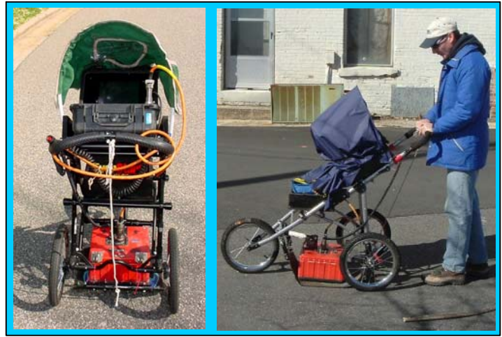
The photographs show the SIR-2000 GPR system equipped with a 400 MHz antenna that were used to conduct the ground penetrating radar investigation at Parcel 79 on January 6, 2010.
