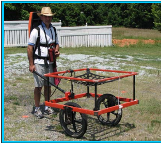
The photograph shows the Geonics EM61 metal detector that was used to conduct the metal detection survey across the proposed Right-of-Way portion of Parcel 79 on December 29, 2009.
