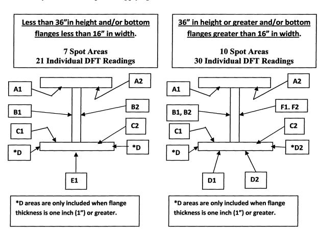
A. Two random adhesion tests (1 test=3 dollies) per span are conducted on interior surfaces in accordance with ASTM D-4541 (Adhesion Pull Test) after the prime coat has been properly cured in accordance with ASTM D-4752 (MEK Rub Test) with no less than a 4
