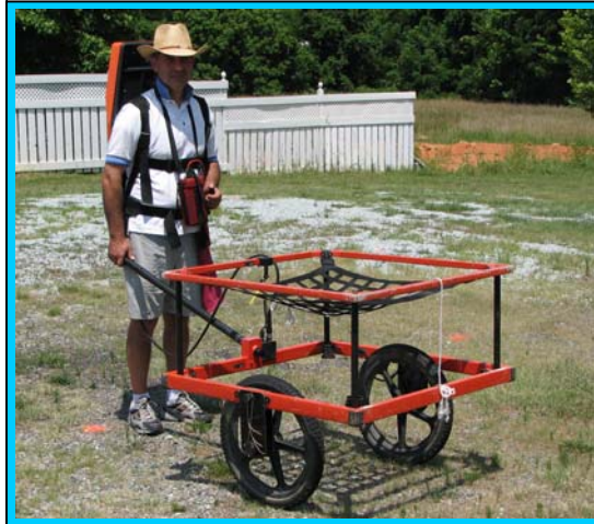
The photograph shows the Geonics EM61 metal detector that was used to conduct the metal detection survey across the proposed Right-of-Way portion of Parcel 119 on May 13, 2010.
