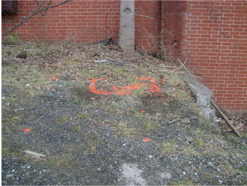
Parcel 4 – Paddy Mountain Lumber Inc., looking northwest. Photo shows approximate marked location of the probable UST near the southeast corner of the building.
