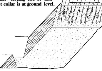
5. Place a 2 inch layer of well rotted sawdust over the roots maintaining a sloping angle.
