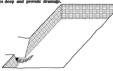
3. Backfill the trench with 2 inches well rotted sawdust. Place a 2 inch layer of well rotted sawdust at a sloping angle at one end of the trench.
