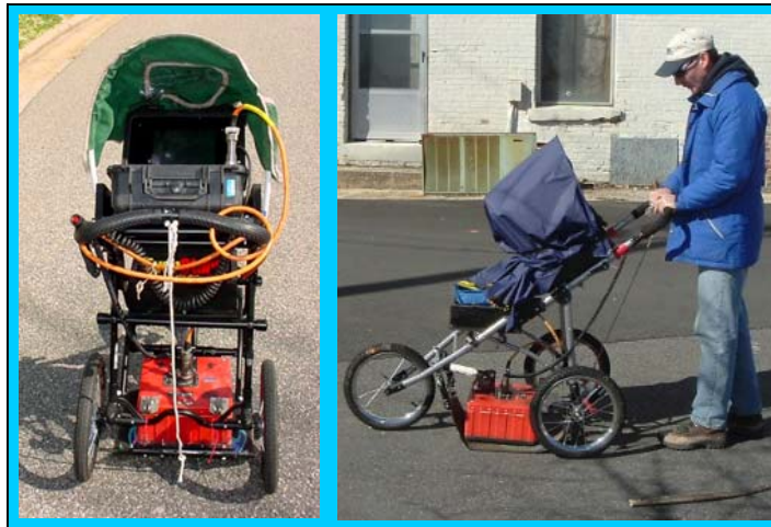
The photographs show the SIR-2000 GPR system equipped with a 400 MHz antenna that were used to conduct the ground penetrating radar (GPR) investigation at the 610 East Elizabeth Street site on July 8, 2010.
