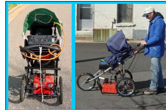
The photographs show the SIR-2000 GPR system equipped with a 400 MHz antenna that were used to conduct the ground penetrating radar investigation at the sites in Winston-Salem, North Carolina. The GPR surveys were conducted during the week of March 15, 2010.
