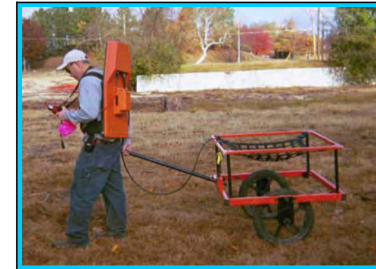
The photograph shows the Geonics EM61 metal detector that was used to conduct the metal detection survey at the sites in Winston-Salem, North Carolina. The EM61 surveys were conducted during the week of March 8, 2010
