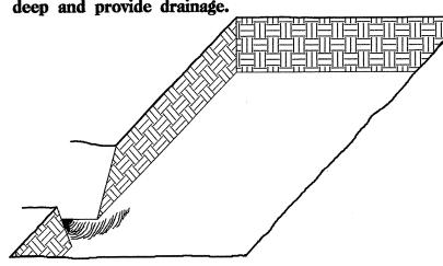
3. Backfill the trench with 50mm well rotted sawdust. Place a 50mm layer of well rotted sawdust at a sloping angle at one end of the trench.
