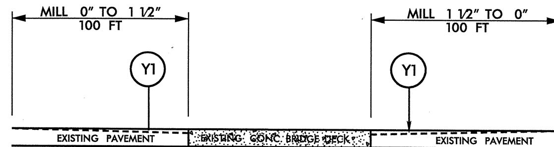
DETAIL A MILLING BRIDGE APPROACHES
