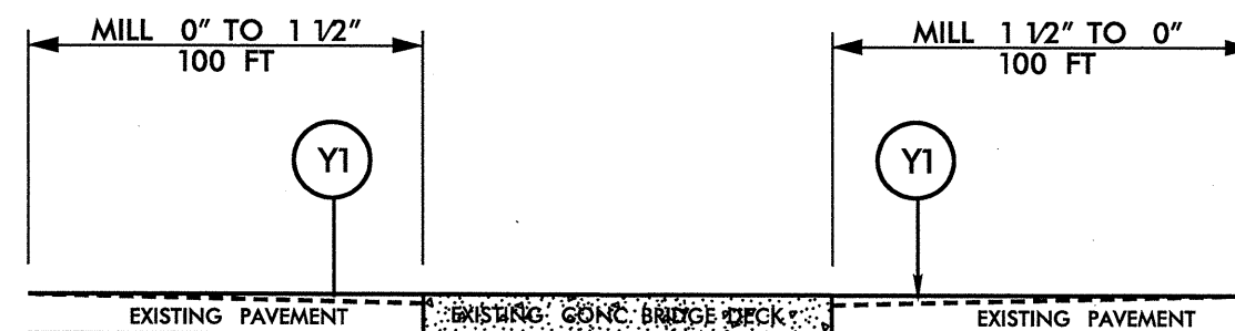
DETAIL A MILLING BRIDGE APPROACHES
