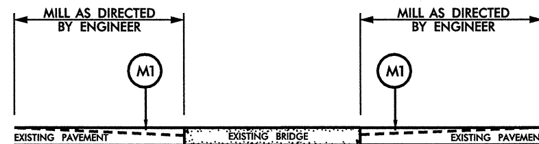
DETAIL 2 MILLING APPROACHES
