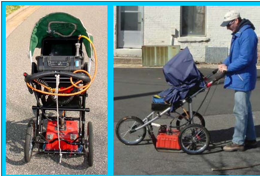
The photographs show the SIR-2000 GPR system equipped with a 400 MHz antenna that were used to conduct the ground penetrating radar investigation at the Jerry Pell property.
