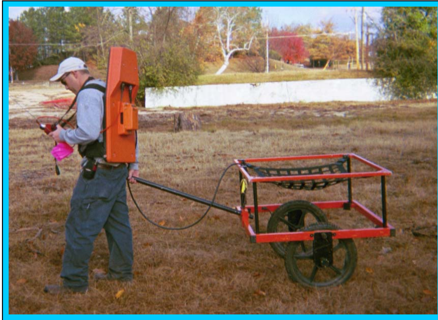
The photograph shows the Geonics EM61 metal detector that was used to conduct the metal detection survey at the Jerry Pell property.
