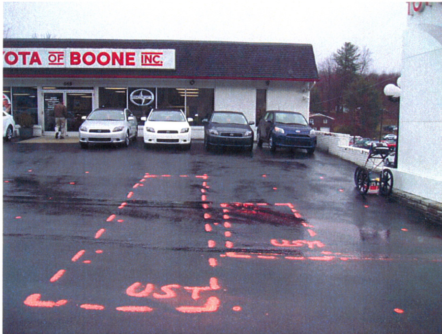
Parcel 51 – Toyota of Boone, looking north UST's: 5' x 24', 4' x 10'
