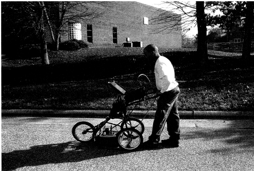
Geophysical Survey Systems SIR-2000 with 400 MHz antenna
