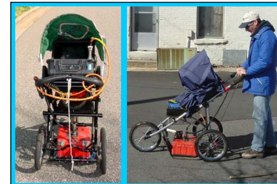
The photos show the SIR-2000 GPR system equipped with a 400 MHz antenna that was used to conduct the ground penetrating radar investigation at the sites in Richmond County, North Carolina.
