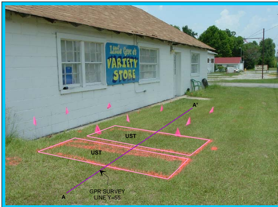
The photograph shows the location of two probable USTs buried approx. 0.75 feet below surface, as suggested by the geophysical results at Parcel 50.
