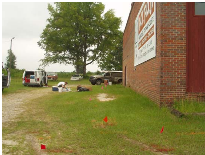
Photograph 2. Parcel 48 looking northwest along side of garage. Potential location of buried metallic UST identified by flags in foreground.
