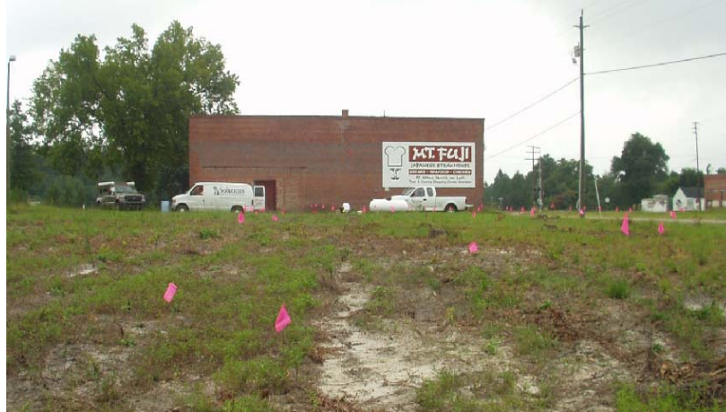
Photograph 3. Parcel 48 looking northeast toward garage (location of soil borings P48B3 through P48B7 identified with orange flags). US Highway 1 is located to the right of the photograph.
