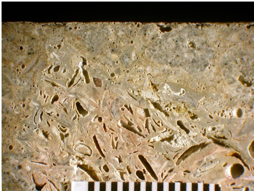
Figure 22. Pores in a coarse aggregate particle near the top surface of Core 137 contain soft, clay-like deposits. Millimeter scale.
