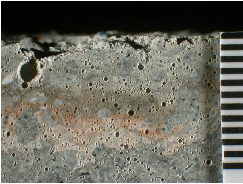
Figure 16. Paste alteration at the outside end of Core 103. Millimeter scale.
