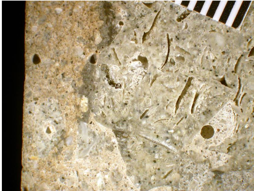
Figure 19. Discolored, carbonated paste at the top of Core 93. Millimeter scale.
