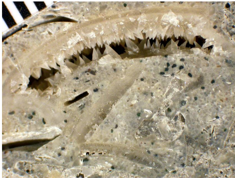
Figure 24. Carbonate crystals line a shell cavity within a limestone coarse aggregate particle.
