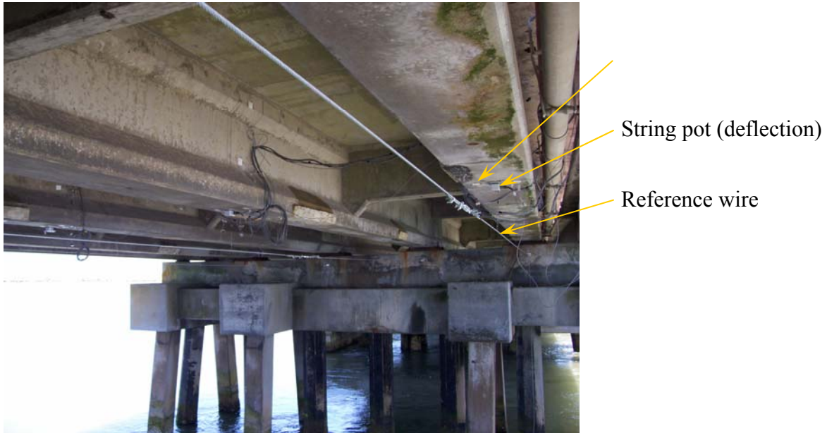
Figure 3. Overall of instrumentation setup.
