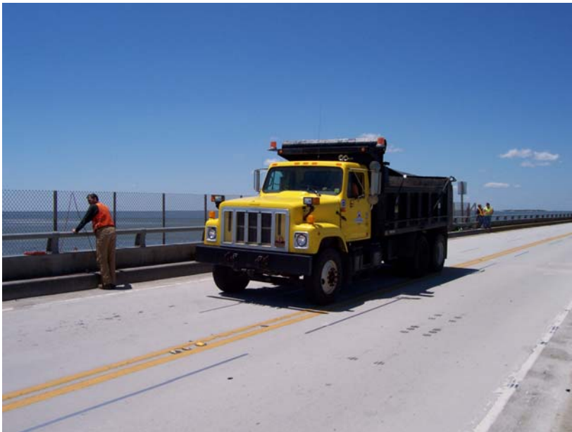
Figure 8. Truck centered over Girder No. 3 (looking north).
