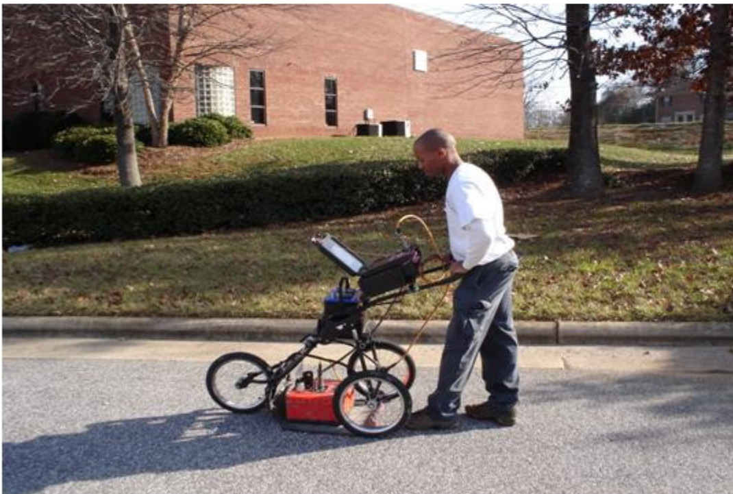
Geophysical Survey Systems SIR-2000 with 400 MHz antenna
