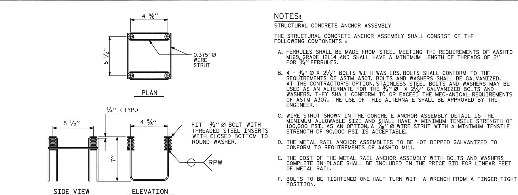
MINIMUM LENGTH OF THREADS IN INSERT (FERRULE): 13/4"
