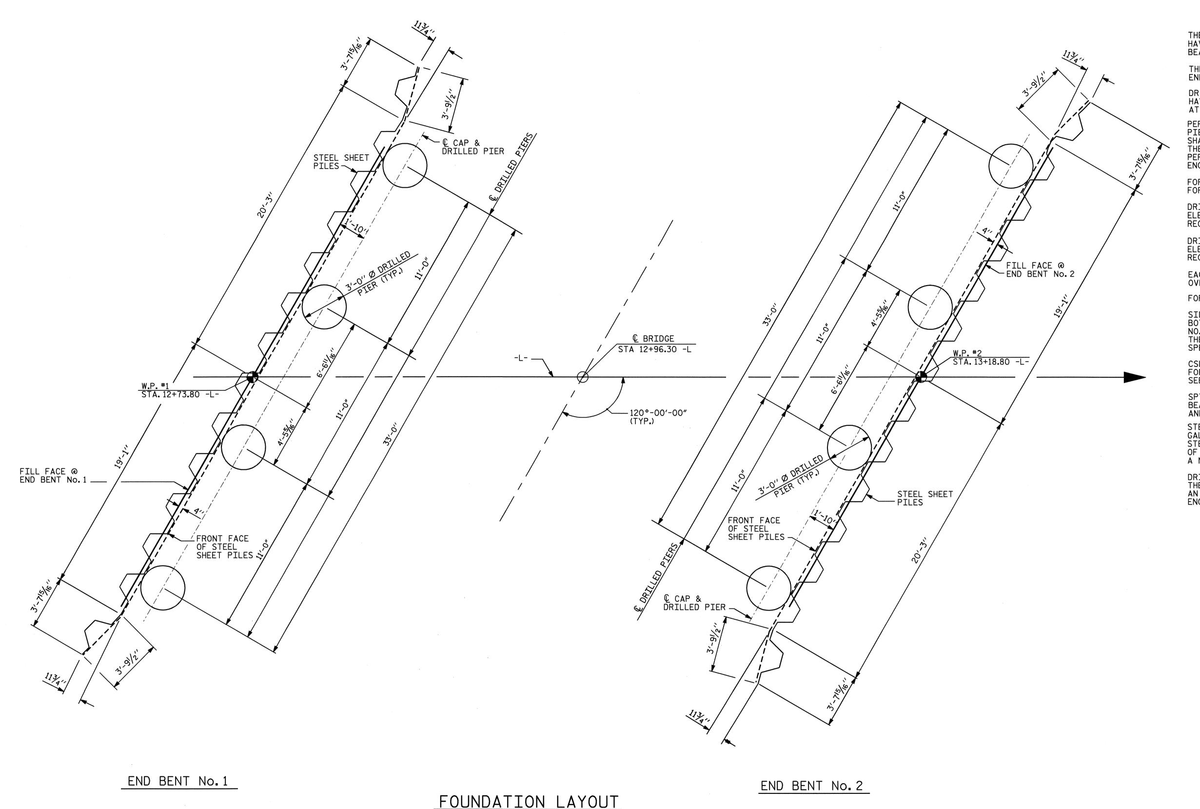
DIMENSIONS LOCATING DRILLED PIERS ARE SHOWN TO THE DRILLED PIER CENTERLINE
