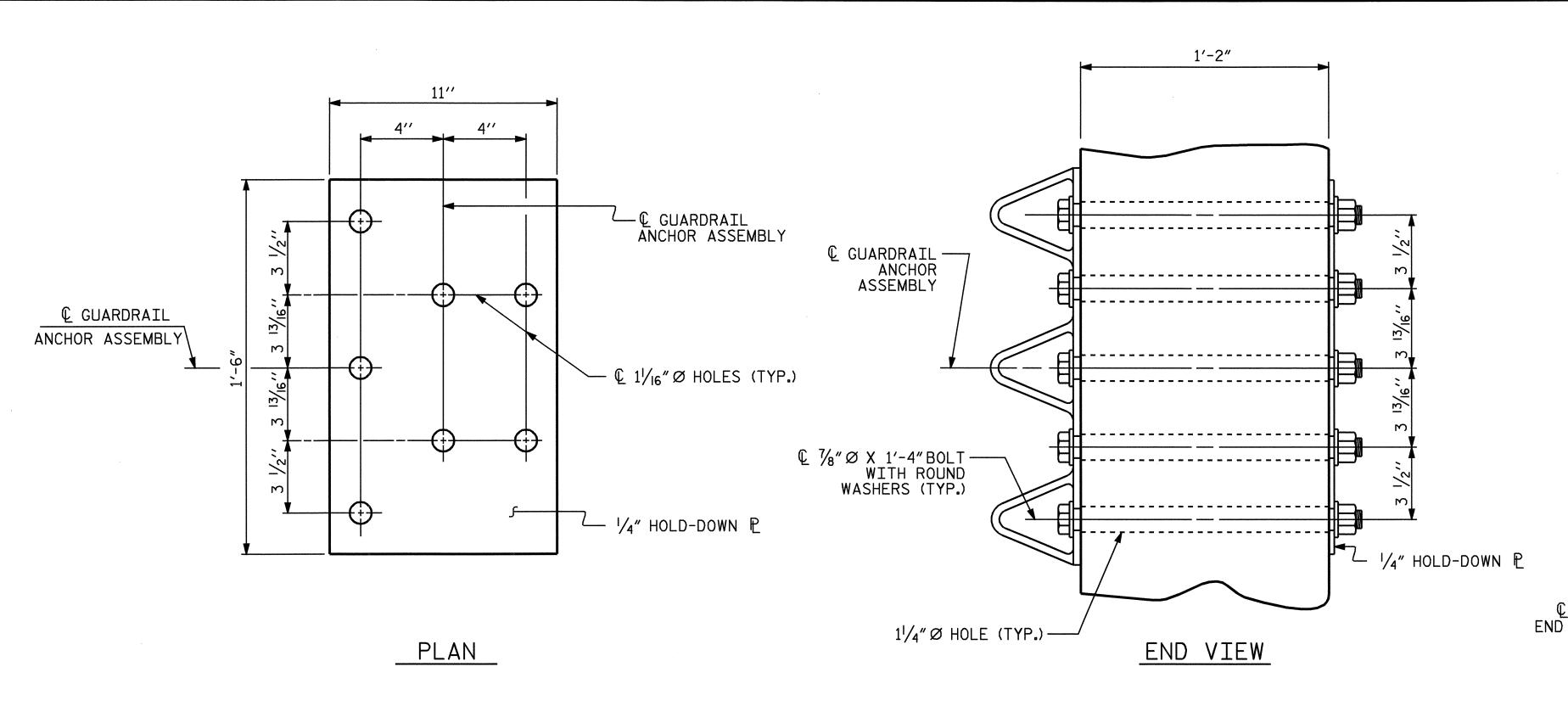
GUARDRAIL ANCHOR ASSEMBLY DETAILS
