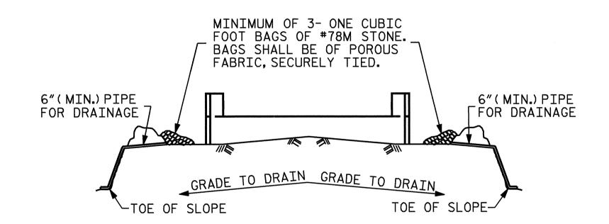
BAGGED STONE AND PIPE SHALL BE PLACED IMMEDIATELY AFTER COMPLETION OF END BENT EXCAVATION. PIPE MAY BE EITHER CONCRETE, CORRUGATED STEEL, CORRUGATED ALUMINUM ALLOY, OR CORRUGATED PLASTIC. PERFORATED PIPE WILL NOT BE ALLOWED.
