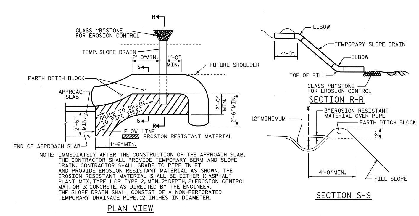
TEMPORARY BERM AND SLOPE DRAIN DETAILS
