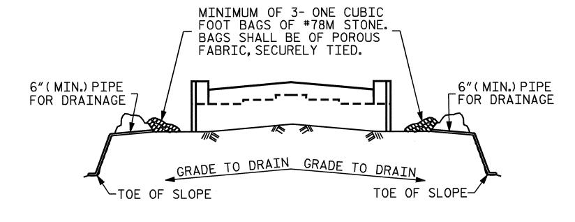
BAGGED STONE AND PIPE SHALL BE PLACED IMMEDIATELY AFTER COMPLETION OF END BENT EXCAVATION. PIPE MAY BE EITHER CONCRETE, CORRUGATED STEEL, CORRUGATED ALUMINUM ALLOY, OR CORRUGATED PLASTIC. PERFORATED PIPE WILL NOT BE ALLOWED.
