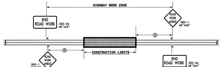
MINIMUM SIGN SPACING POSTED SPEED LIMIT (8) (M.P.H.) ≤ 50 500' ≥ 55 1000'
