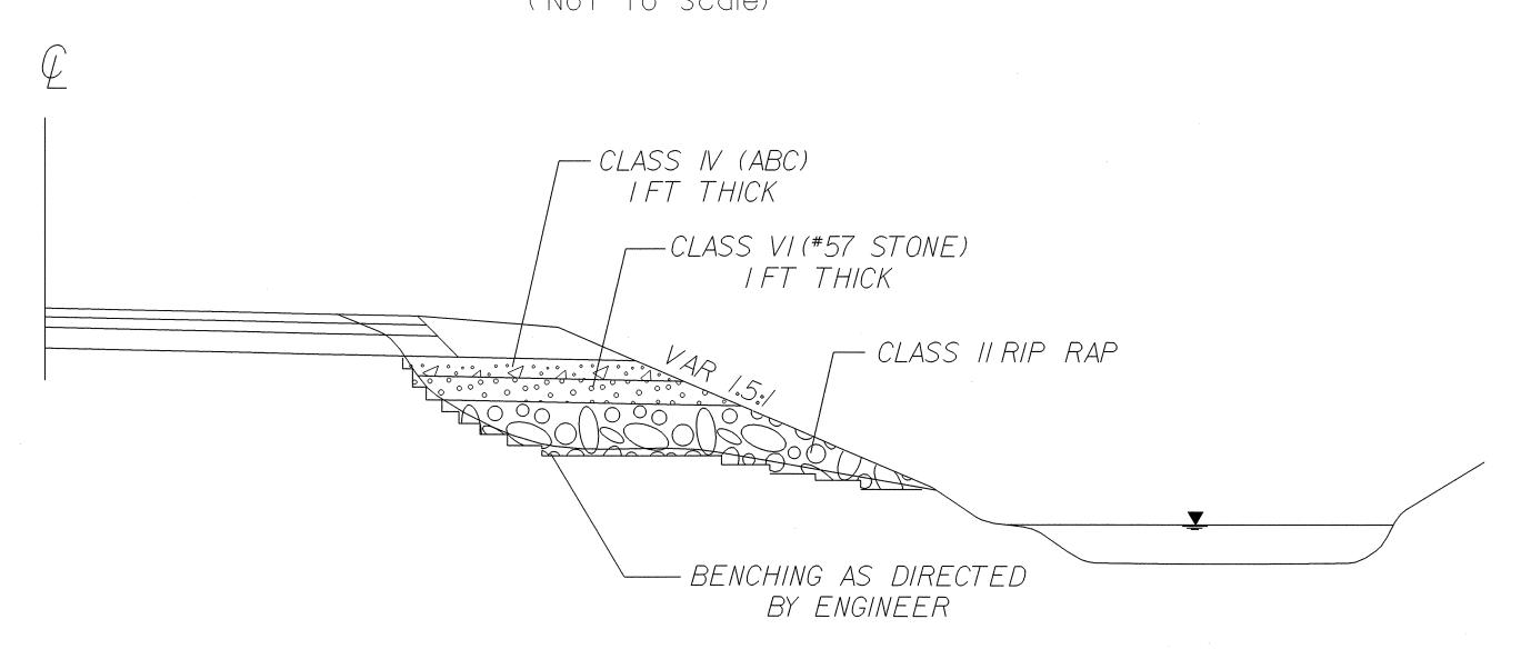
SELECT MATERIAL, CLASS IV = 230 TONS SELECT MATERIAL, CLASS VI = 190 TONS PLAIN RIP RAP, CLASS II = 215 TONS FILTER FABRIC = 470 SY
