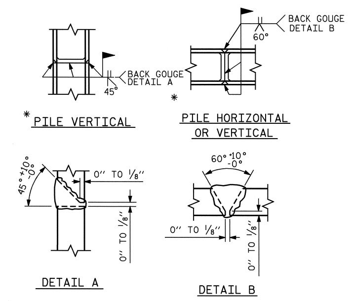
\*POSITION OF PILE DURING WELDING.
