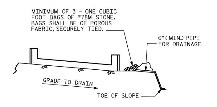
BAGGED STONE AND PIPE SHALL BE PLACED IMMEDIATELY AFTER COMPLETION OF END BENT EXCAVATION. PIPE MAY BE EITHER CONCRETE, CORRUGATED STEEL, CORRUGATED ALUMINUM ALLOY, OR CORRUGATED PLASTIC. PERFORATED PIPE WILL NOT BE ALLOWED.
