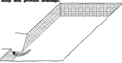
3. Backfill the trench with 2 inches well rotted sawdust. Place a 2 inch layer of well rotted sawdust at a sloping angle
