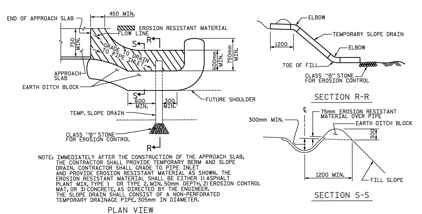
TEMPORARY BERM AND SLOPE DRAIN DETAILS
