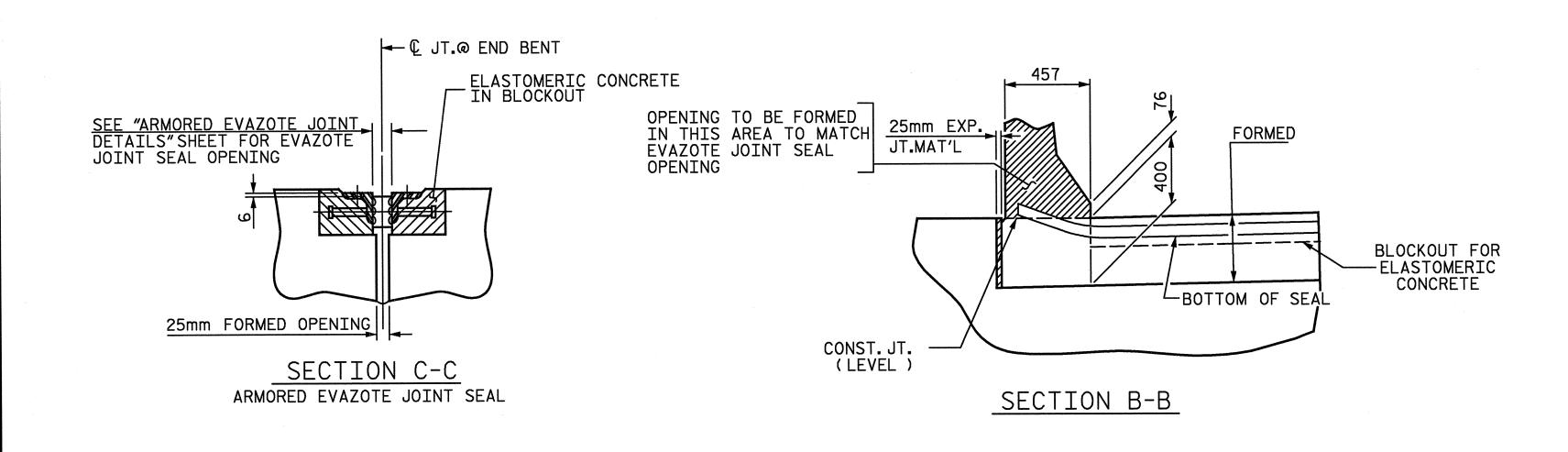
JOINT SEAL DETAILS @ END BENT
