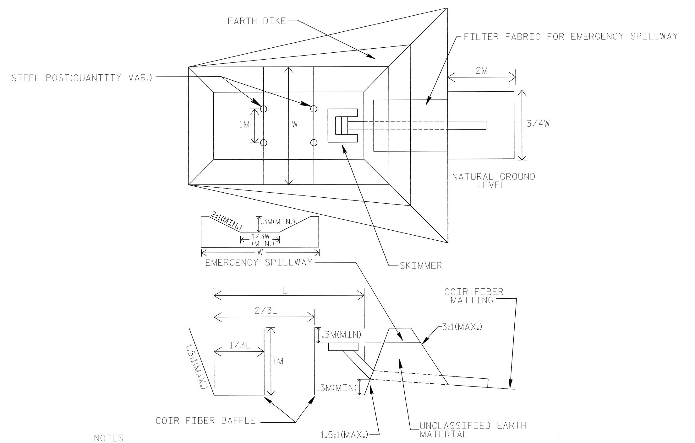
ALL COIR FIBER SHALL BE CONSTRUCTED WITH 700 G/M<sub>2</sub> COIR, NORTH AMERICAN GREEN C-125BN COIR BLANKET, OR EQUIVALENT SPECIFICATIONS.
