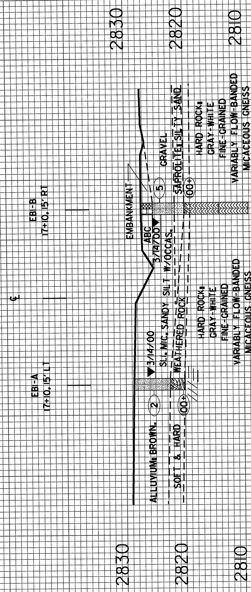
CROSS SECTION THROUGH BENT ONE
