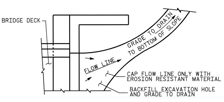
NOTE: IF THE APPROACH SLAB IS NOT CONSTRUCTED IMMEDIATELY AFTER THE BACKFILLING OF THE END BENT EXCAVATION, GRADE TO DRAIN TO THE BOTTOM OF THE SLOPE AND PROVIDE EROSION RESISTANT MATERIAL, SUCH AS FIBERGLASS ROVING OR AS DIRECTED BY THE ENGINEER TO PREVENT SOIL EROSION AND TO PROTECT THE AREA ADJACENT TO THE STRUCTURE. THE CONTRACTOR WILL BE REQUIRED TO REMOVE THESE MATERIALS PRIOR TO CONSTRUCTION OF THE APPROACH SLAB.
