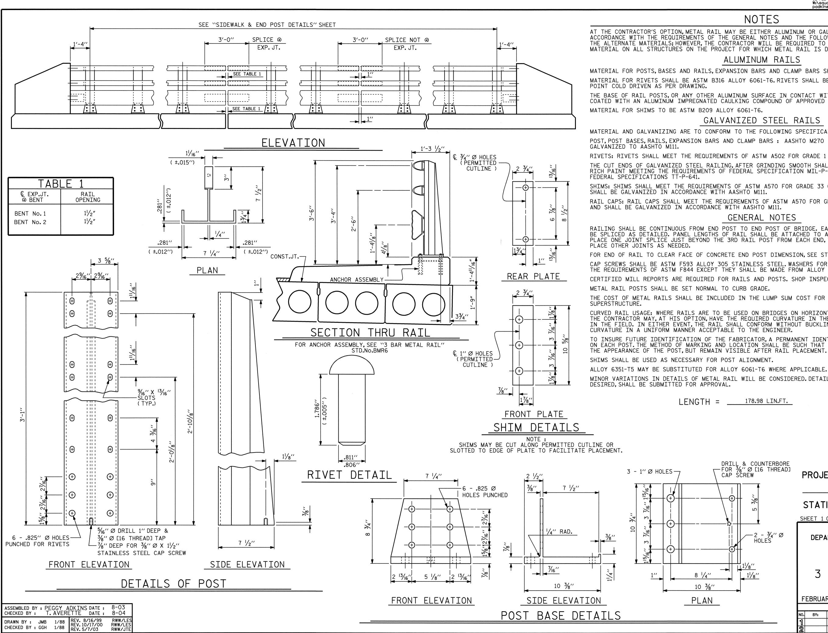
AT THE CONTRACTOR'S OPTION, METAL RAIL MAY BE EITHER ALUMINUM OR GALVANIZED STEEL IN ACCORDANCE WITH THE REQUIREMENTS OF THE GENERAL NOTES AND THE FOLLOWING SPECIFICATIONS FOR THE ALTERNATE MATERIALS; HOWEVER, THE CONTRACTOR WILL BE REQUIRED TO USE THE SAME RAIL MATERIAL ON ALL STRUCTURES ON THE PROJECT FOR WHICH METAL RAIL IS DESIGNATED.
