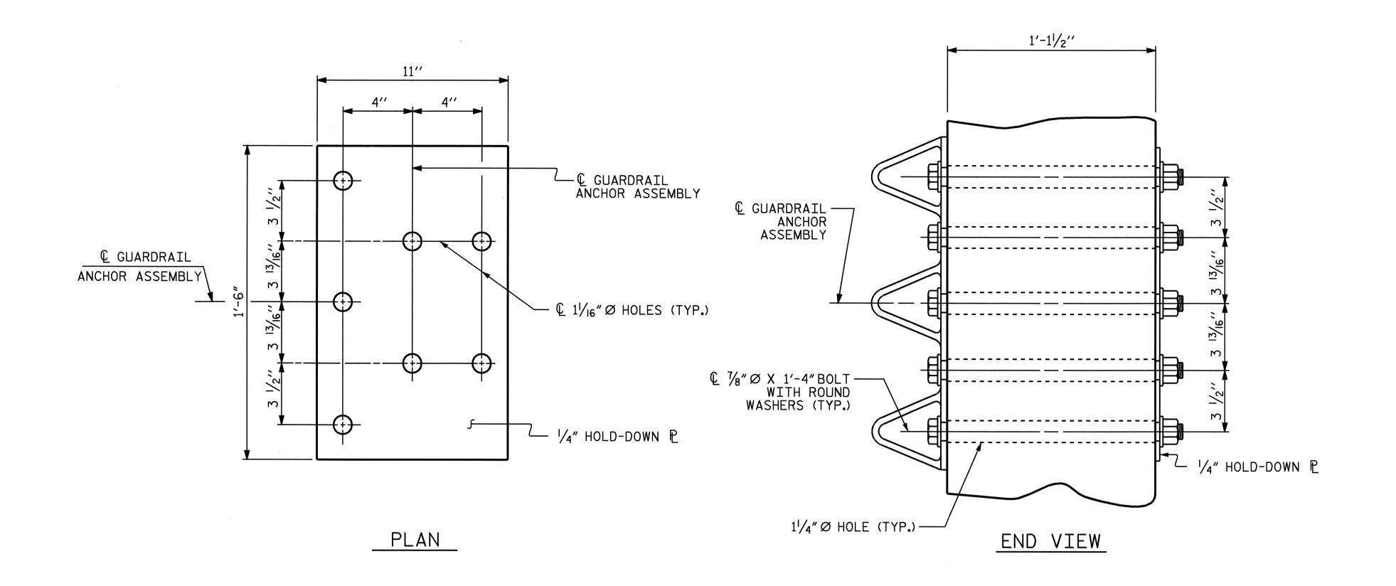
GUARDRAIL ANCHOR ASSEMBLY DETAILS
