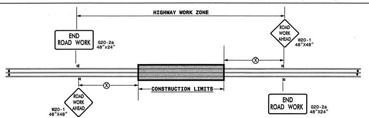
RECOMMENDED MINIMUM SIGN SPACING POSTED SPEED LIMIT (X) (M.P.H.) ≤ 50 500' ≥ 55 1000
