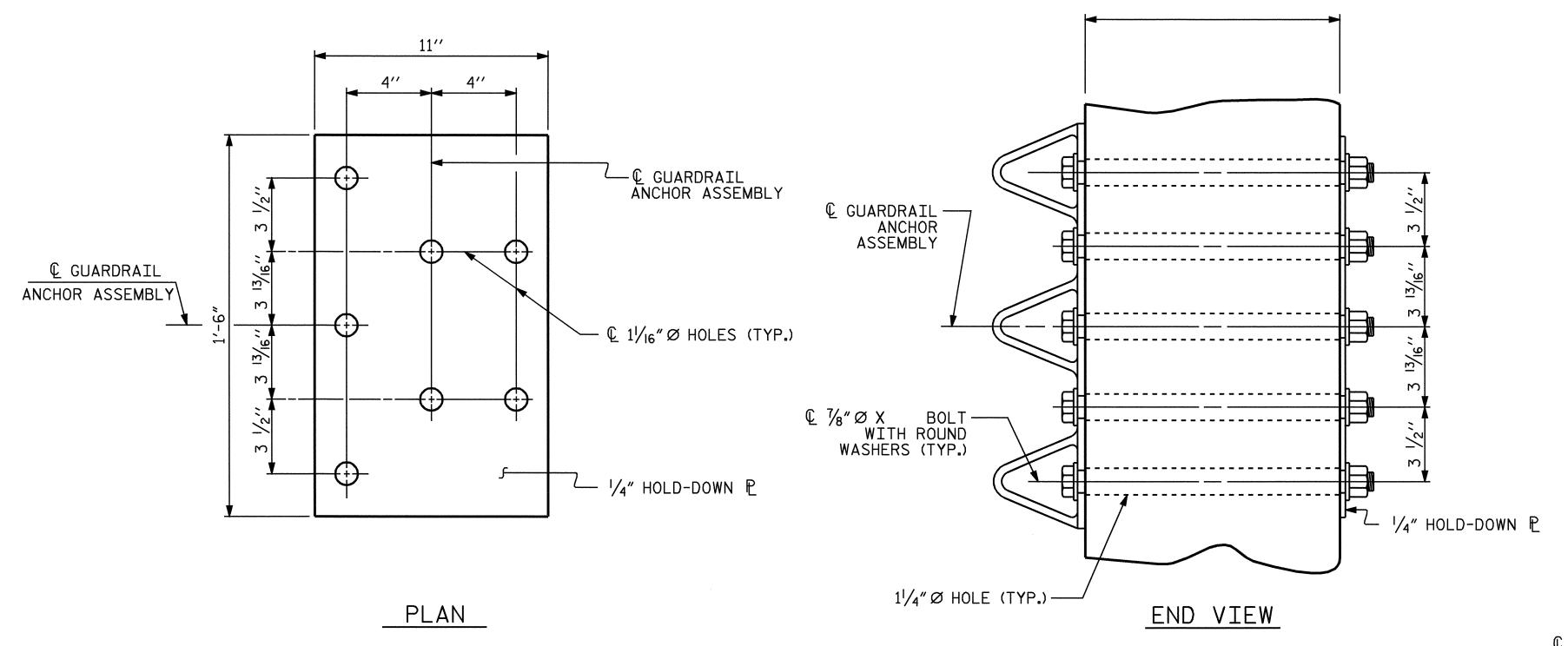
GUARDRAIL ANCHOR ASSEMBLY DETAILS
