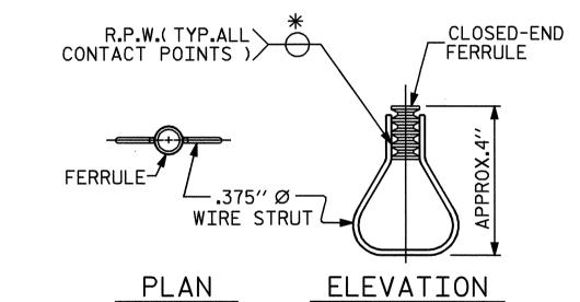
STRUCTURAL CONCRETE INSERT
