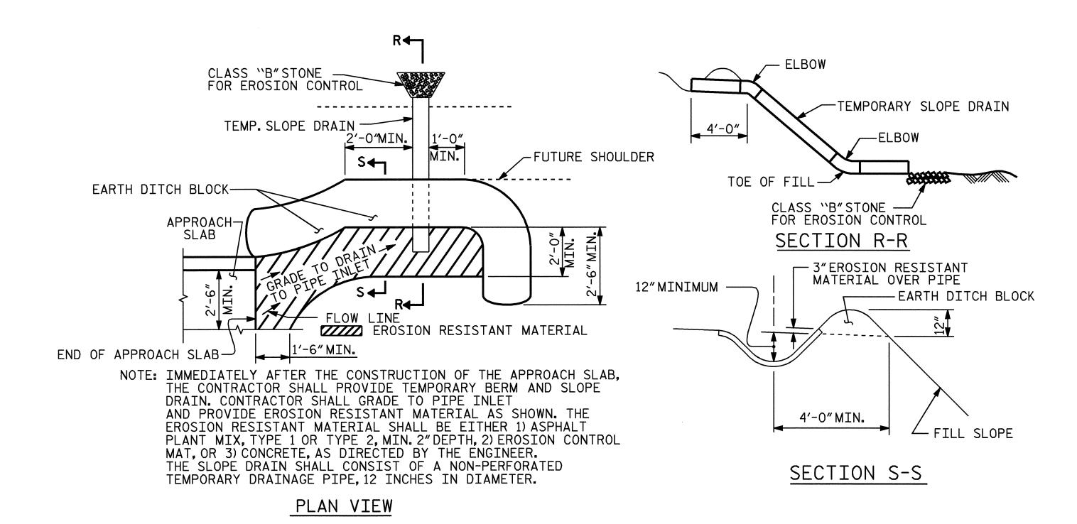
TEMPORARY BERM AND SLOPE DRAIN DETAILS
