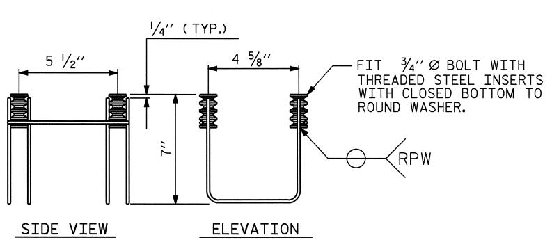
MINIMUM LENGTH OF THREADS IN INSERT (FERRULE): 13/4"
