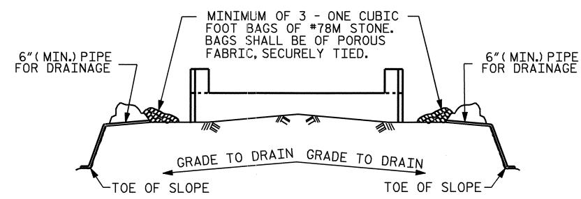
BAGGED STONE AND PIPE SHALL BE PLACED IMMEDIATELY AFTER COMPLETION OF END BENT EXCAVATION. PIPE MAY BE EITHER CONCRETE, CORRUGATED STEEL, CORRUGATED ALUMINUM ALLOY, OR CORRUGATED PLASTIC. PERFORATED PIPE WILL NOT BE ALLOWED.
