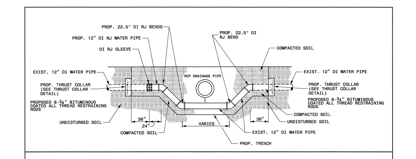
WATER PIPE CROSSING STORM DRAIN
