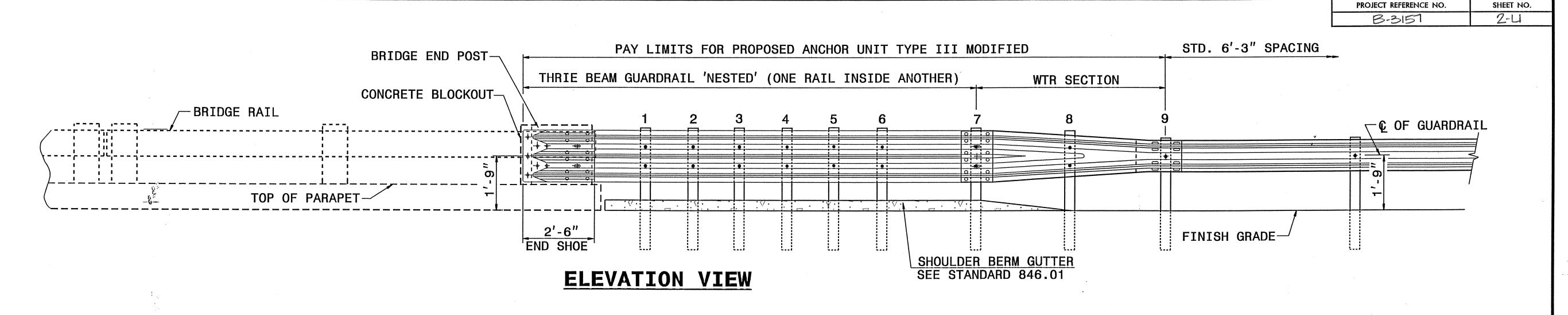
\*THE DISTANCE FROM END OF BRIDGE RAIL TO CENTER LINE OF THE FIRST POST SHOULD BE 111/2" IF CONCRETE BACKWALL IS NOT PRESENT. \*\*POST NOT REQUIRED FOR SKEW ANGLES GREATER THAN 150° OR LESS THAN 30° UNLESS OTHERWISE DIRECTED BY THE ENGINEER.
