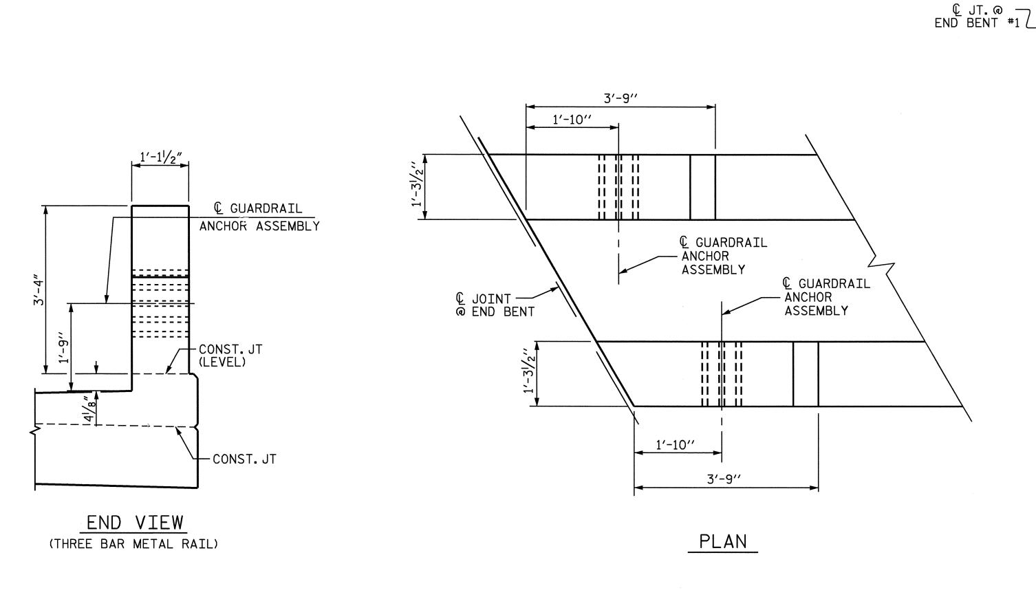
LOCATION OF GUARDRAIL ANCHOR AT END POST
