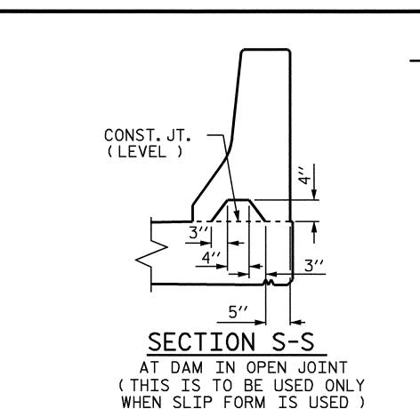
THE BARRIER RAIL IN A CONTINUOUS UNIT SHALL NOT BE CAST UNTIL ALL SLAB CONCRETE IN THE UNIT HAS BEEN CAST AND HAS REACHED A MINIMUM COMPRESSIVE STRENGTH OF 3,000 PSI.
