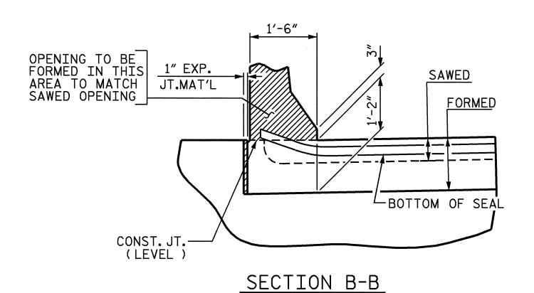
JOINT SEAL DETAILS @ END BENT (FOR BARRIER RAIL)
