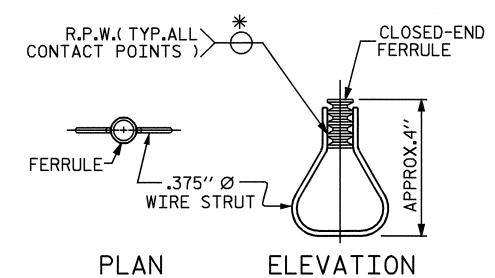
\* EACH WELDED ATTACHMENT OF WIRE TO FERRULE SHALL DEVELOP THE TENSILE STRENGTH OF THE WIRE.
