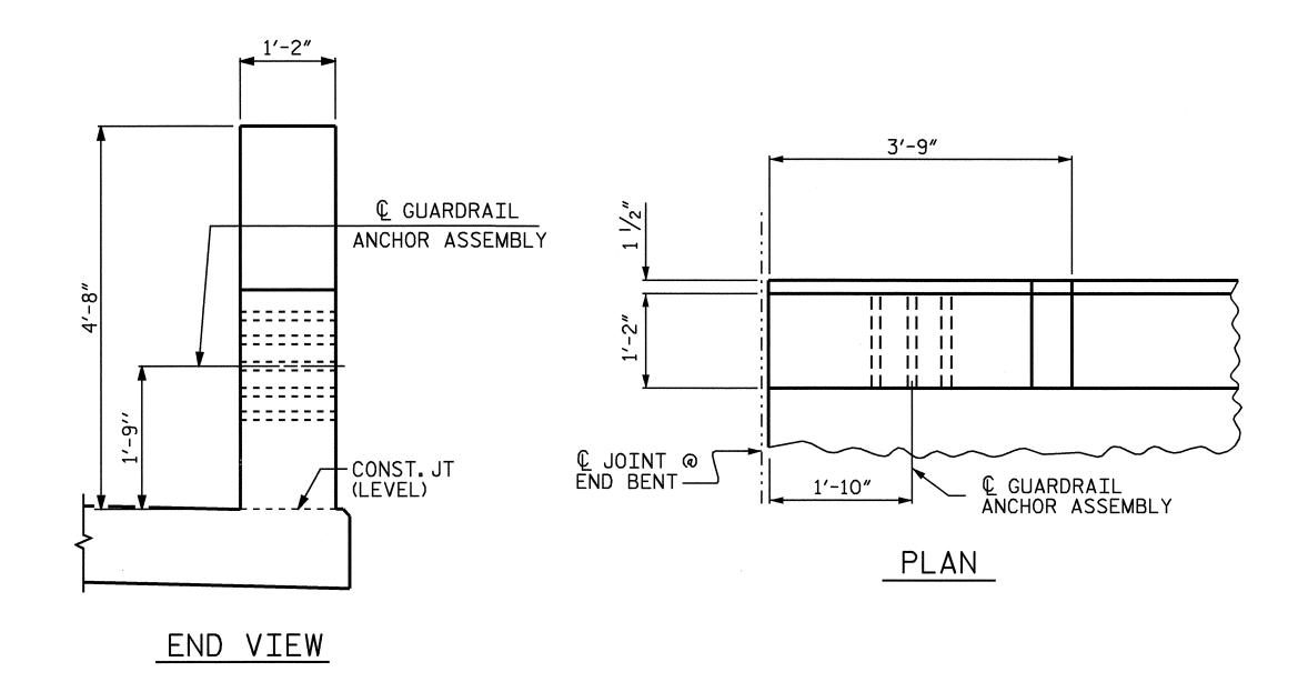
LOCATION OF GUARDRAIL ANCHOR AT END POST
